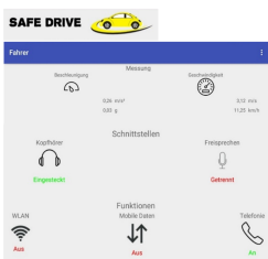
Fig. 1: Interruption of mobile phone functions when a certain speed is exceeded
